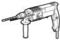
Hammer drill (with a drill bit of 8 mm)
